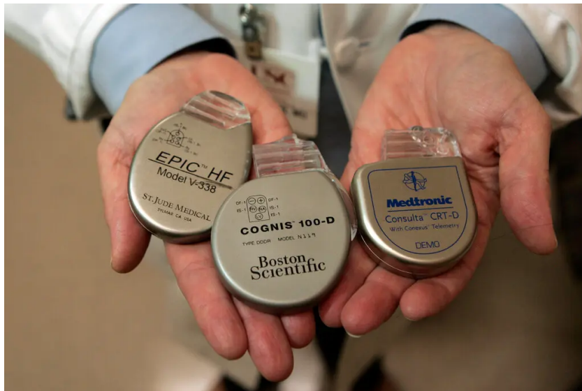
Implantable cardioverter defibrillators can deliver a shock to the wearer’s heart in the case of sudden cardiac arrest. Ann Johansson for The New York Times
